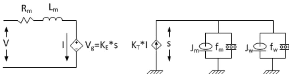
Here  $J_w$  and  $f_w$  are the inertia and the friction of the wheel respectively. Now, we can re-draw our electrical equivalent:
