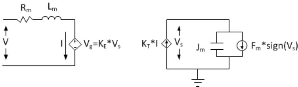
As you can see, I've replaced the speed with voltage ( $V_s$ ), all the components with their electrical equivalent and the mechanical ground with the electrical one. This latest step is not really relevant. In fact, when you replace the mechanical ground, you can replace it with any constant voltage node. Just make sure you keep some absolute and constant reference around for the mechanical portion.
