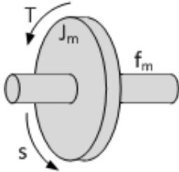
Let's use our newly acquired knowledge and draw a mechanical schematic representation of it! We have two mechanical components to consider: the rotating mass and the friction. These two components are connected to the same shaft, so the one end of the two symbols are connected together:
