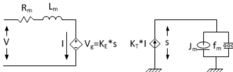
At first it looks quite a bit complicated, but in fact it really isn't: it only makes the electrical/mechanical conversion in the motor explicit. It shows both the controlled voltage source (which is the conversion in the mechanical  $\rightarrow$  electrical direction) and the controlled torque source (which is the conversion in the electrical  $\rightarrow$  mechanical direction).
