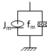
There are two things missing: the source of the mechanical energy and the mechanical load. If we model the motor alone, the load is simple: we don't have it. The source isn't that complex either: it is the torque converted by the motor. This torque is acting between the shaft and the housing of the motor, and as we've discussed before, we assume that the motor housing is stationary:
